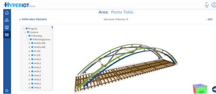
Figure 4 - BIM Model from Tekla Structures to HyperIoT
